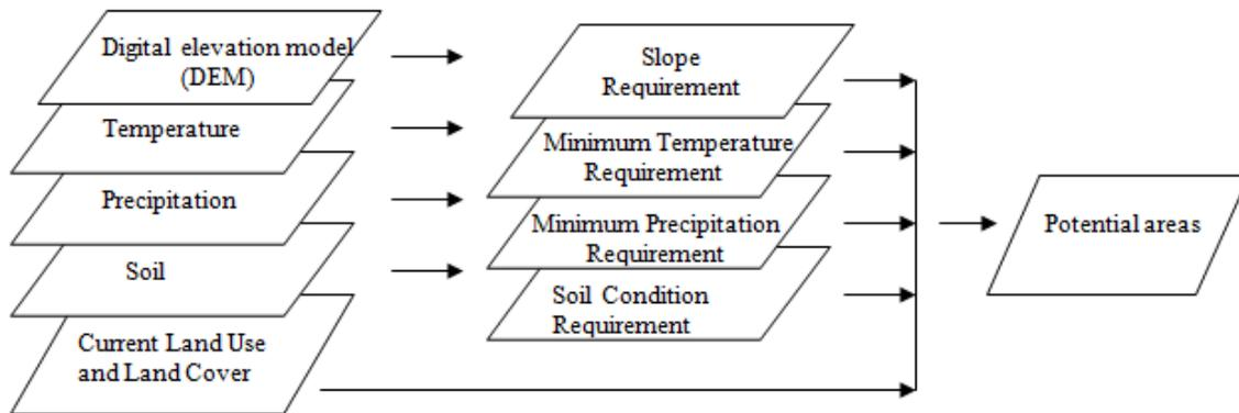
Figure 5. A cartographic model of using GIS to identify potential areas for rice production
